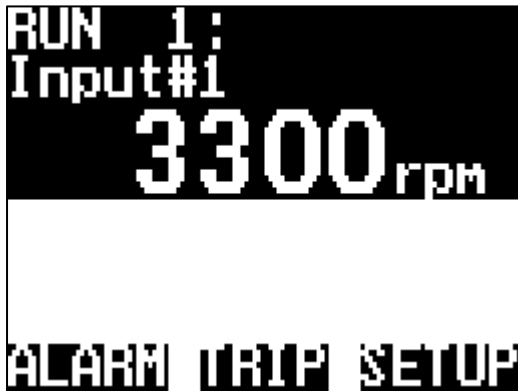
When the alarm point is reached e.g.: over 3000rpm the line will FLASH notifying you of the alarm point.
