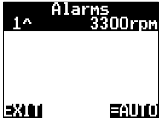
In the example above Line 1 is ^ over the alarm set point. If it was below it would show 1v. You have 3 options:
