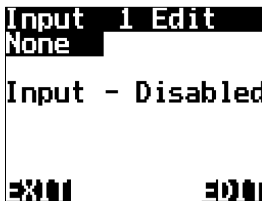
After selecting your input pressing the EDIT button allows you to enable/disable the port
