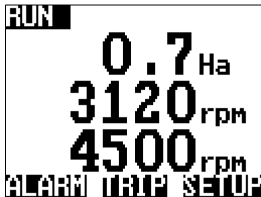
When you now EXIT back to the front screen the order of lines have been changed Line 1 – HA, Line 2 – Shaft 1, Line 3 – Shaft 2
