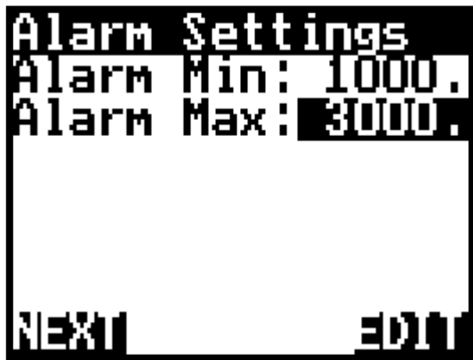
Wizard or manual alarm points. Example of a Shaft Alarm set at Min of 1000RPM & Max of 3000RPM
