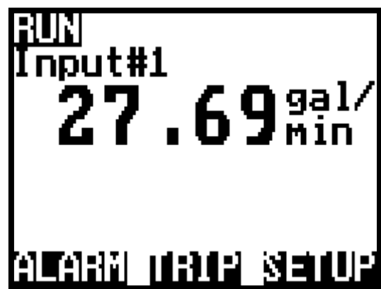
Example : 1 UP monitoring a flow meter in gal/min
