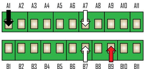
Figure 46: Jackal ports capable of accepting analog sensor inputs. Black is **GROUND**, Red is **POWER** and white is **SIGNAL**. NOTE: do not use any other Ground or Power on the Jackal or vehicle for sensors
