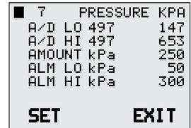
Figure 24: Pressure calibration screen The number immediately to the right of **A/D LO** and **A/D HI** is the live A/D reading. Numbers to the far right are the stored values for the calibration point.
