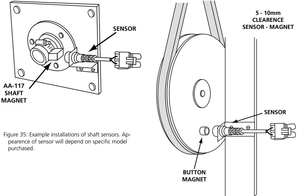
Figure 35: Example installations of shaft sensors. Appearance of sensor will depend on specific model purchased.
