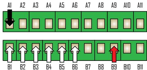
Figure 44: Jackal ports capable of accepting 3 wire 'Reed' sensor inputs. Black is **GROUND**, Red is **POWER** and white is **SIGNAL**. NOTE: do not use any other Ground or Power on the Jackal or vehicle for sensors
