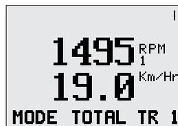
Figure 40: Example of main screen when configured as an Airseeder Surveillance Monitor
