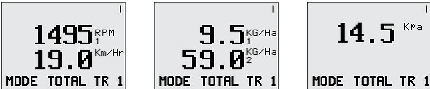
Figure 41: Example of main screen and secondary information screens as the **MODE** button is pressed when configured as an Airseeder monitor as described in this section
