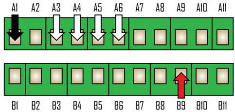
Figure 47: Jackal ports capable of accepting Bin / Tank Level sensor inputs. Black is **GROUND**, Red is **POWER** and white is **SIGNAL**. NOTE: do not use any other Ground or Power on the Jackal or vehicle for sensors
