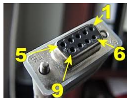
DB9 Female Pinout: Pin 2 RX | Pin 3 TX | Pin 5 GND
