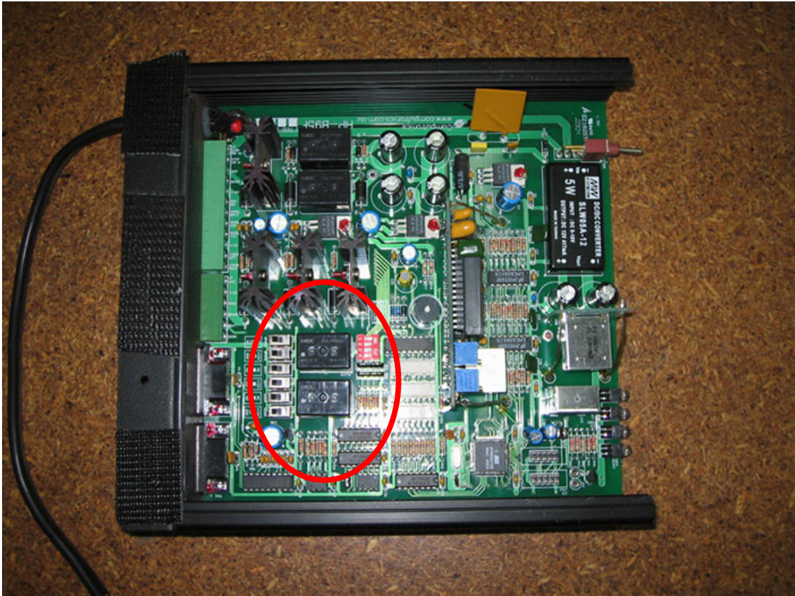
DIP switches and setup switches position on the PCB
