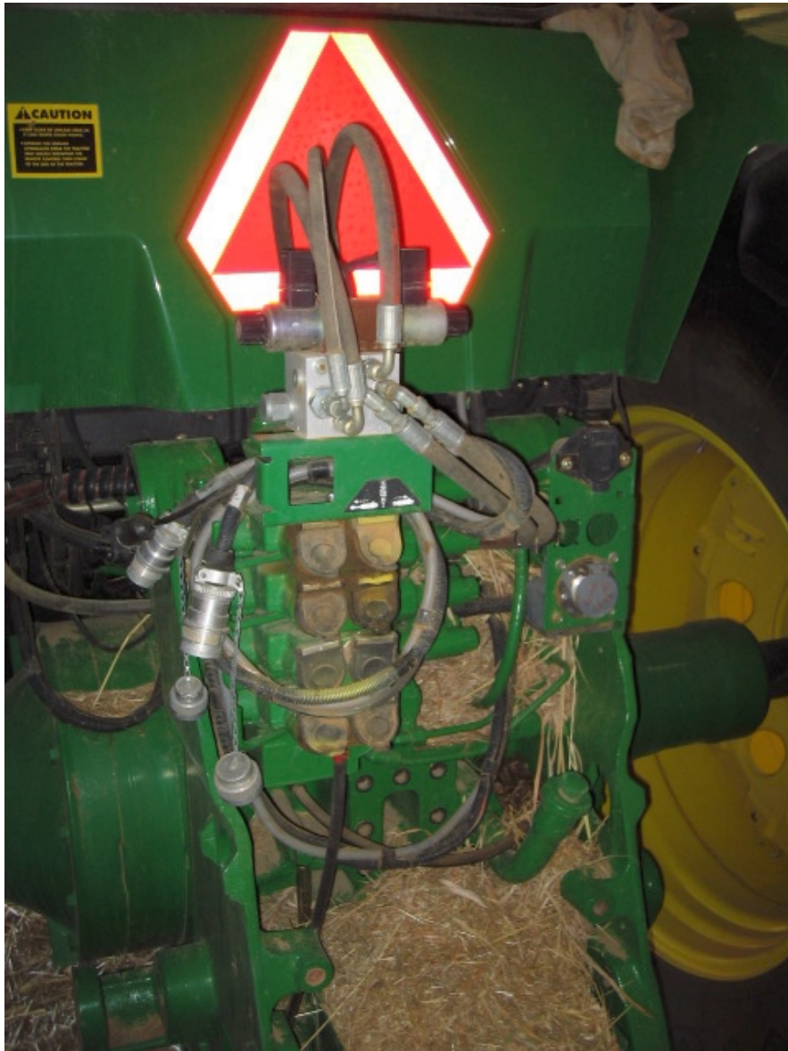
Figure – Power beyond stack
