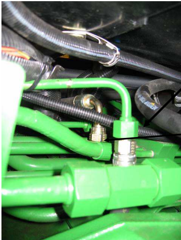
Figure - Load sense between cab and power beyond
