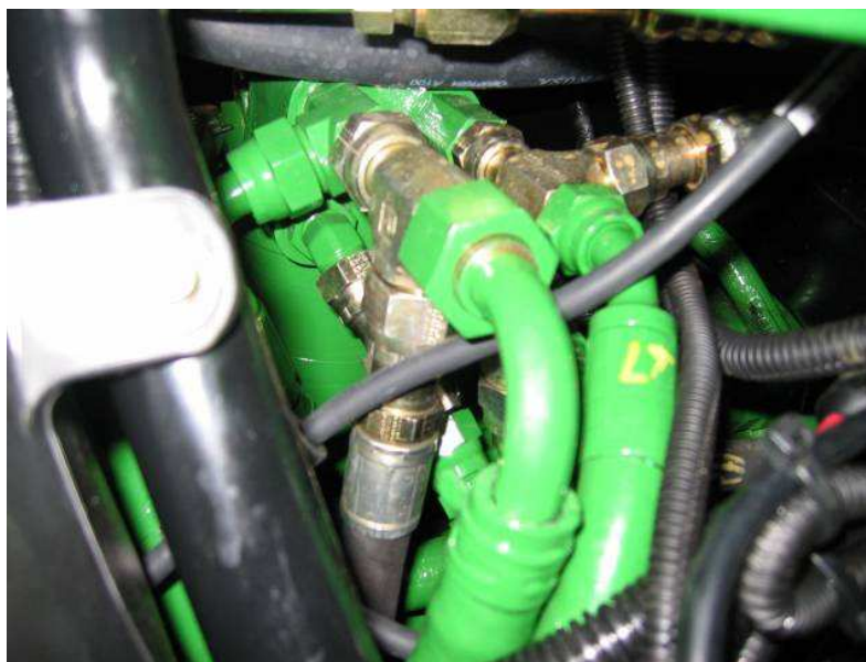
Figure - Tees into system at steering valve
