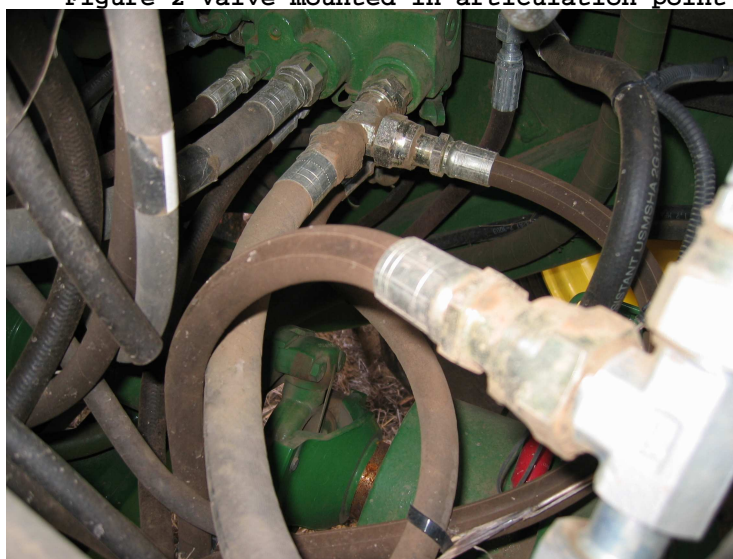
Figure 3- Showing "Tee's" into hoses for pressure and tank
