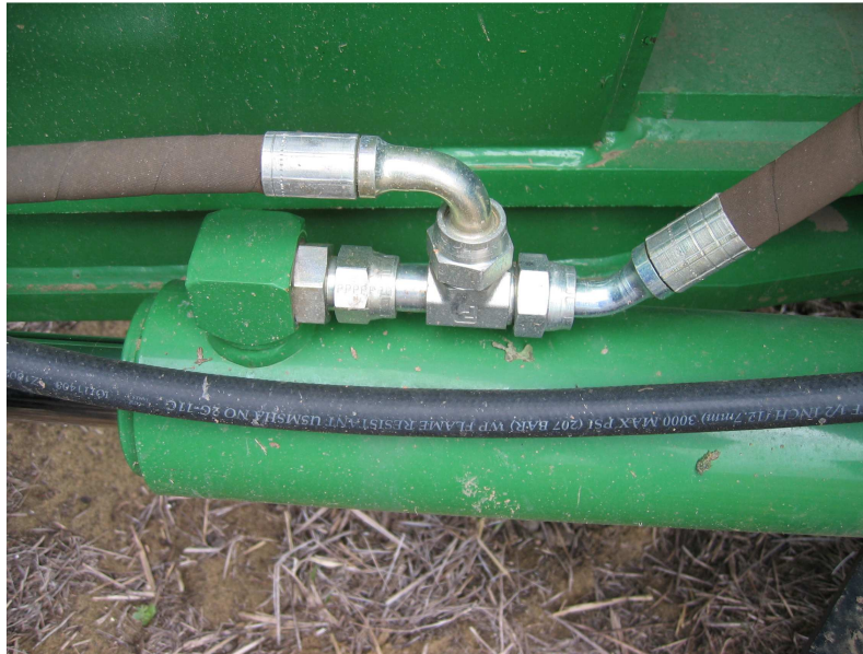
Figure 5- Teeing into the steering rams
