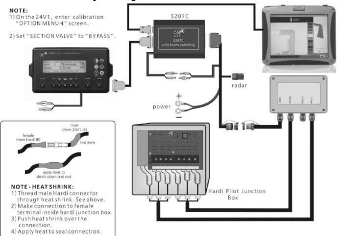
Inside the Hardi Pilot junction box, there are a series of female utilux terminals that come from the external valves and sensors. They plug into the male utilux terminals as shown in the picture below.
