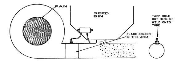
Mount the sensor box in close proximity to the fan out of direct weather exposure and connect the airline cut to length to the pressure fitting.
