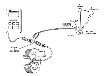
The 1037 MECHANICAL STANDBY connected to any mechanical device that is moved from one position to another (eg. engage lever).
