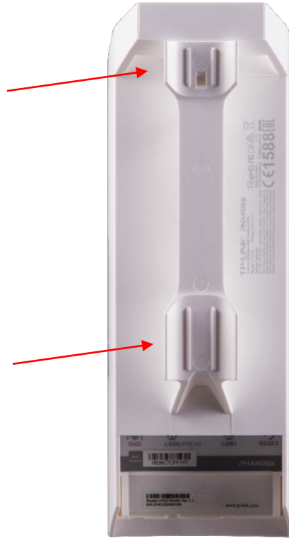
Figure 23: Applying the gaskets to the feet of the access point
