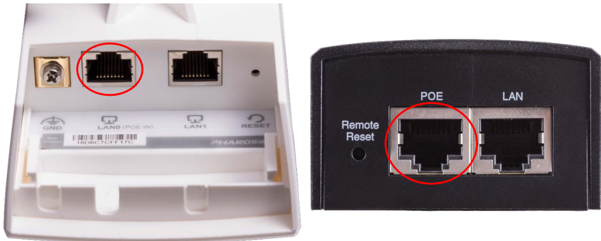
Figure 21: Access point Ethernet connection
