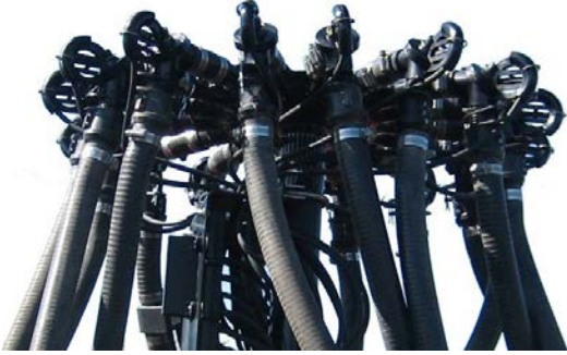
Figure 9: 90-degree flow sensors installed on a manifold
