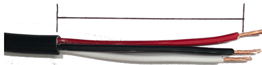
Cable should be trimmed to a minimum of 70mm for easier install in junction box
